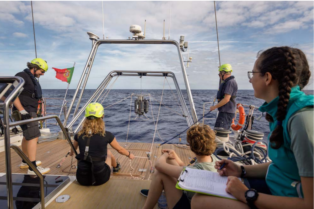
Positioning the water sampling rosette requires skill, as the ocean waves set the valuable device swinging—and in windy weather, the boat can also roll dramatically. Protected from injury by steel-toed shoes and a helmet, marine biologist Hedy Aardema (centre) uses rope hoists to stabilise the rosette, which she then carefully manoeuvres into the sea.
