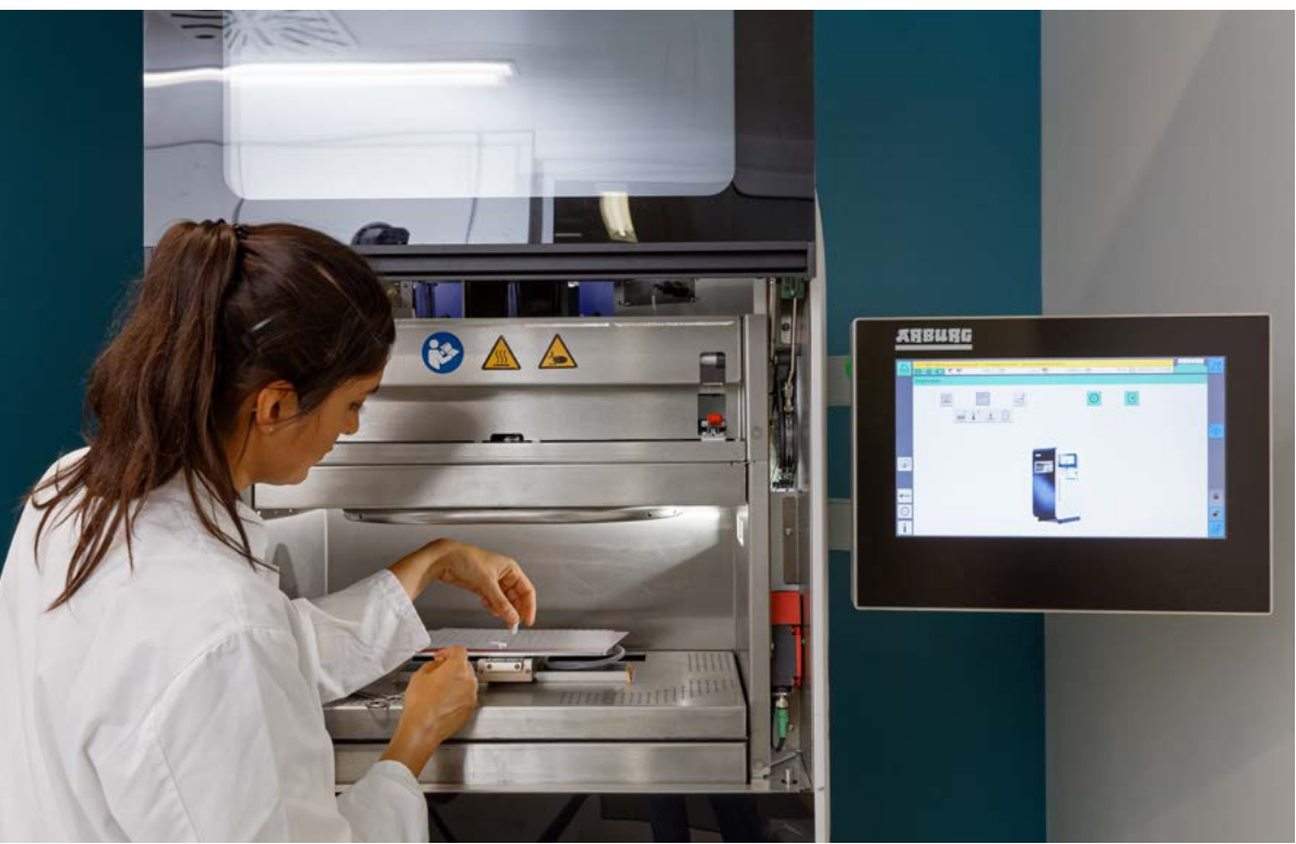
The large 3D printer (shown in full size on page 68, at right) can fabricate implants and bone structures that will later dissolve in the body.
