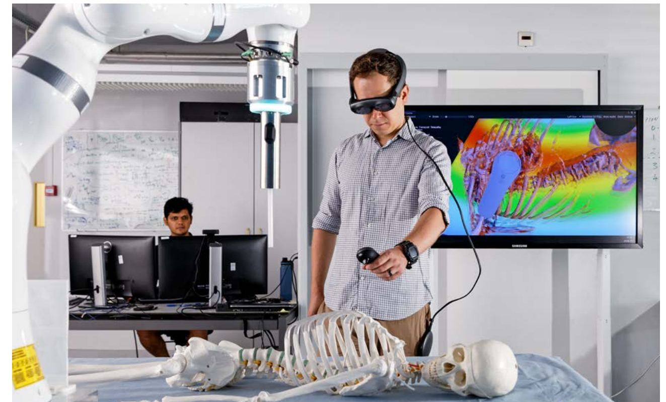
The various robotic components developed are already well aligned: the medical "joystick" detects where on the body a surgical intervention is necessary, and the surgeon, wearing 3D goggles, views a virtual 3D model constructed on the basis of CT scans.
