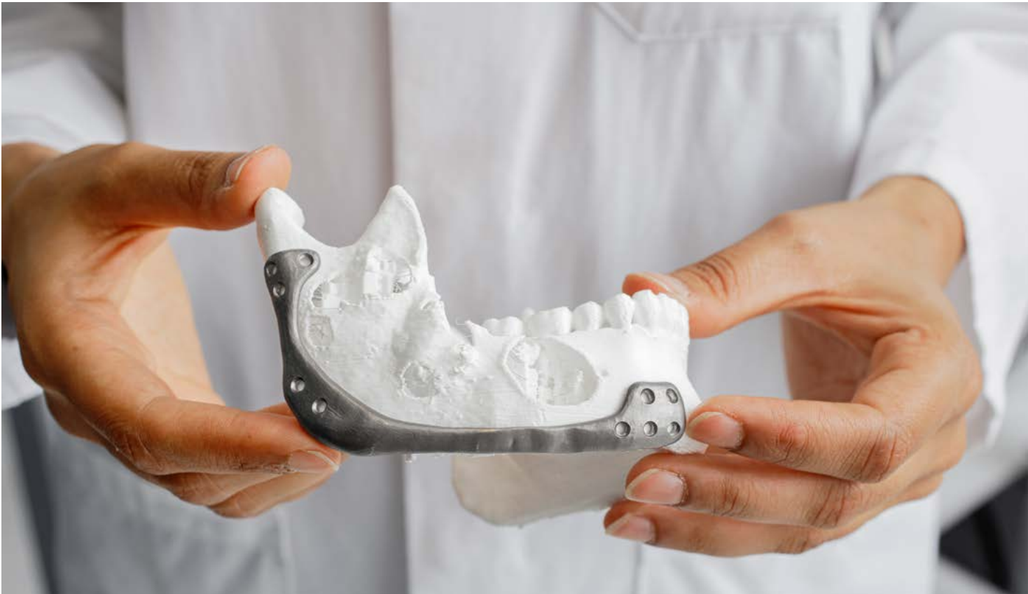
Florian Thieringer, the new co-leader of MIRACLE II, wants to develop personalised bone implants that can be inserted in minimally invasive procedures. In the photograph: a titanium jawbone implant inserted through the patient's oral cavity to stabilise a damaged jawbone.
